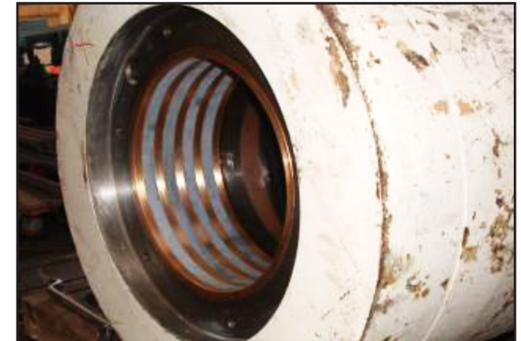
Replaceable bearing bands installed.
