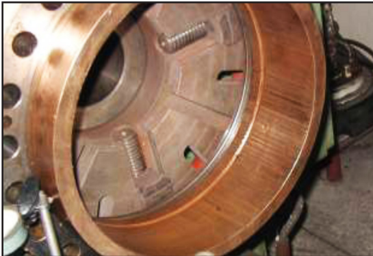
Damaged bronze bearing.
